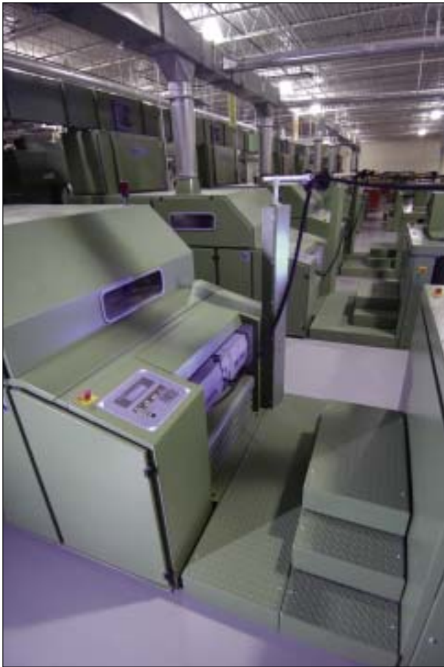
Three of Patrick Yarns' total of 17 Trützschler carding lines.
