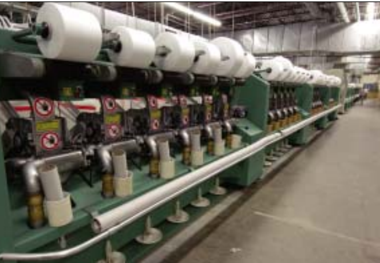
Dref spinning is used to make engineered core yarns and filtration media.
