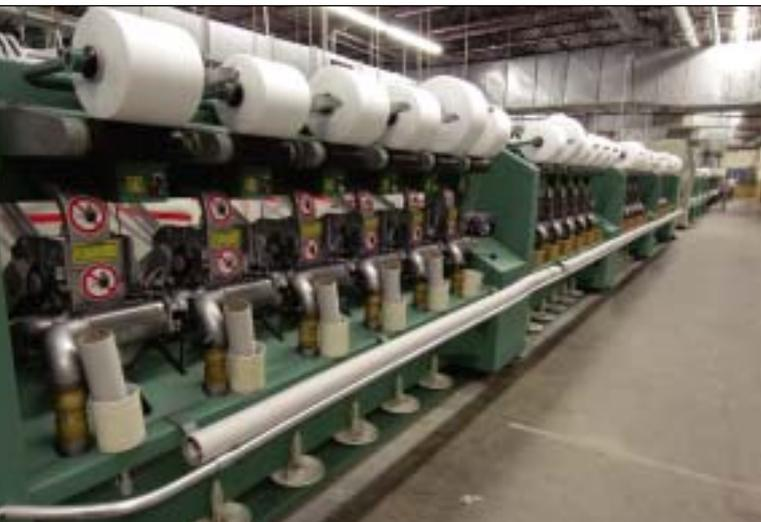
*Dref spinning is used to make engineered core yarns and filtration media.*
